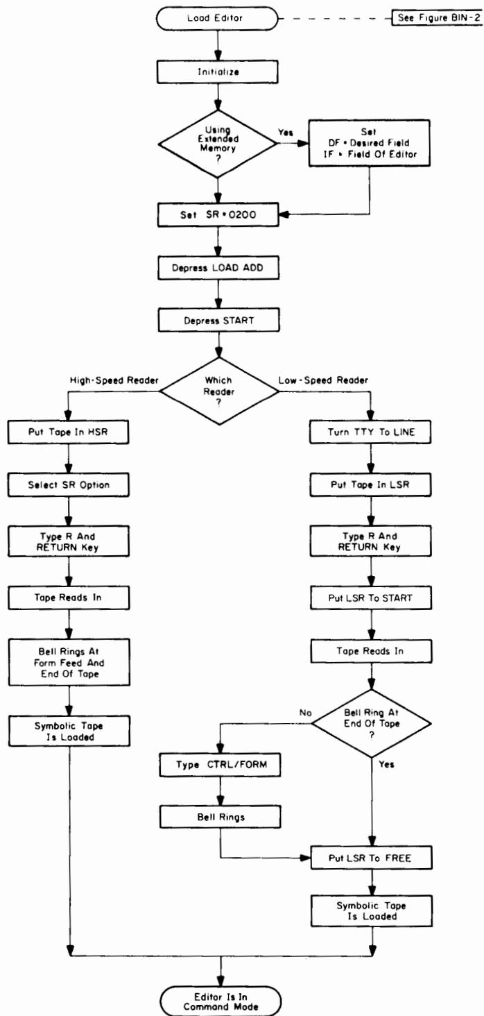
Figure EDIT-3 Loading a Symbolic Tape Using Editor
