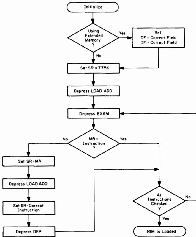
Figure RIM-2 Checking the RIM Loader
