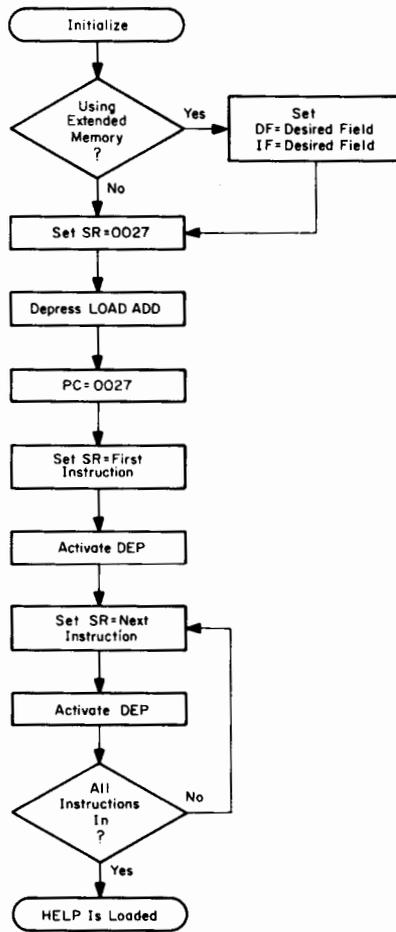
Figure HELP-1 Loading the HELP Loader
