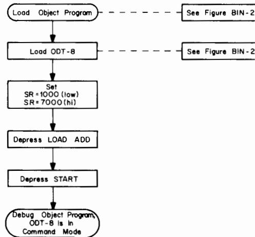
Figure ODT-1 Loading and Executing ODT-8
