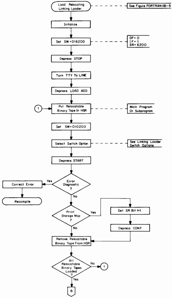
Figure FORTRAN(8K)-6 Loading Relocatable Binary Tapes Using the Relocating Linking Loader
