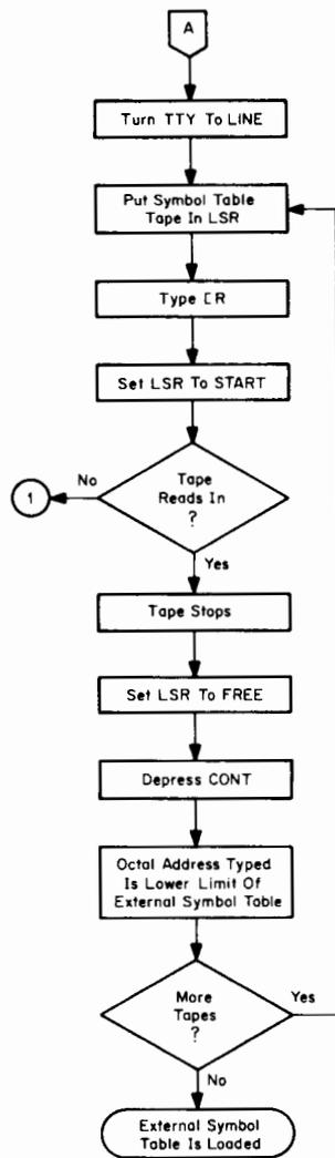
Figure DDT-2 Loading External Symbol Table Tapes (LSR Only)
