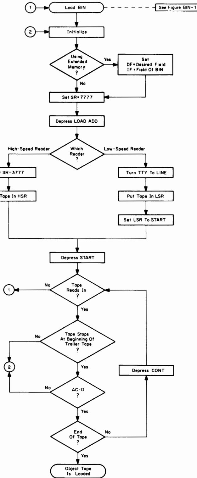
Figure BIN-2 Loading A Binary Coded Object Tape Using BIN
