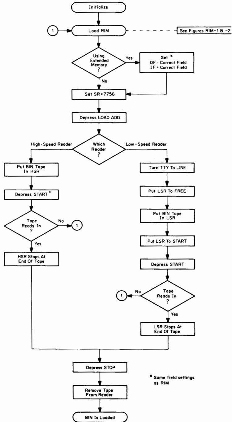
Figure BIN-1 Loading the BIN Loader
