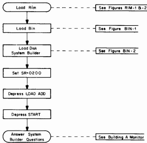
Figure DISK-1 Loading the Disk System Builder
