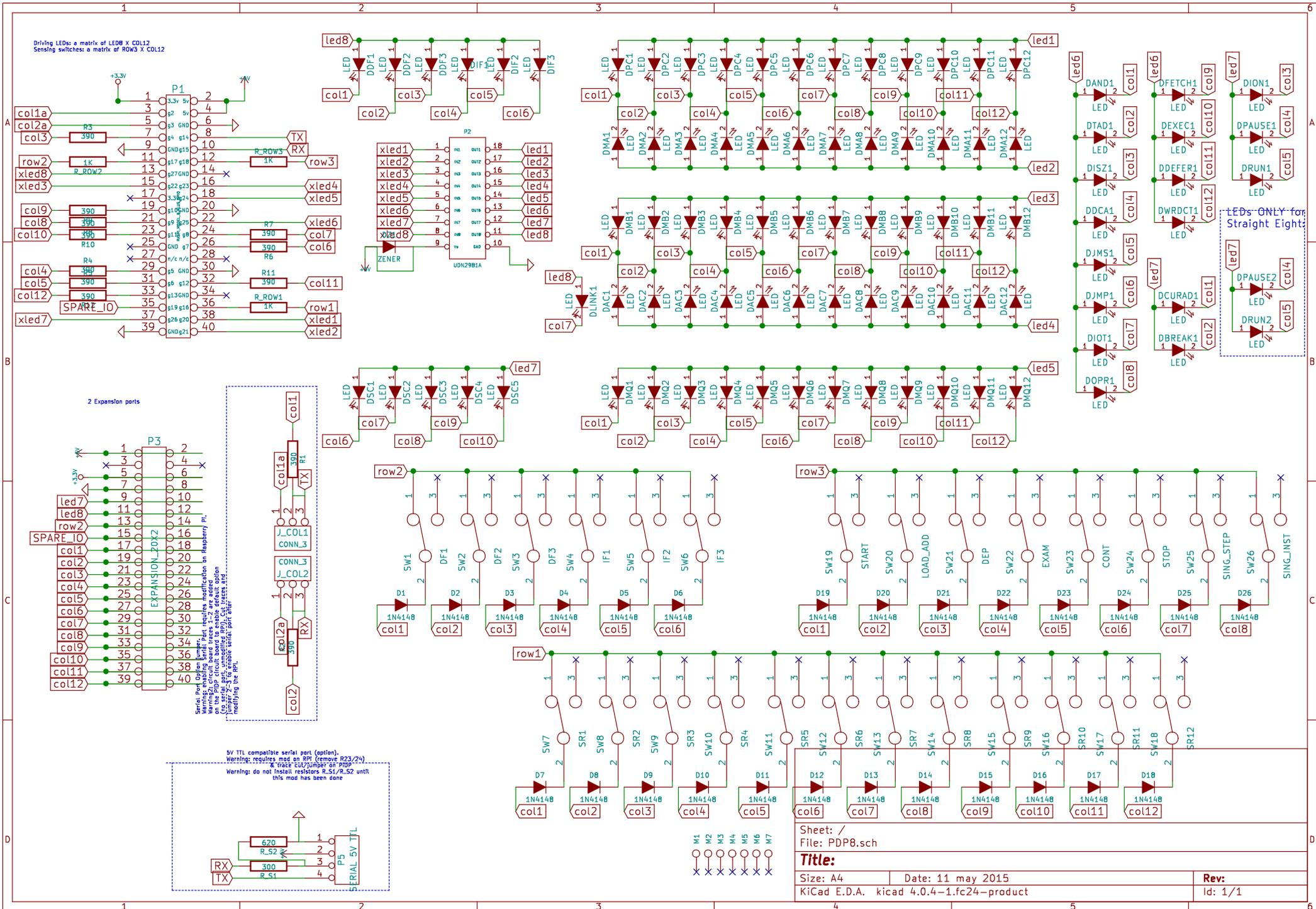
Driving LEDs: a matrix of LED8 X COL12
